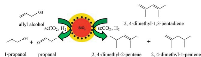
Scheme 1 Illustration of Pd(0) nanocatalysts on SiO 2 particles with a cross-linked polystyrene coating and hydrogenation of 2,4-dimethyl-1,3-pentadiene and allyl alcohol.
